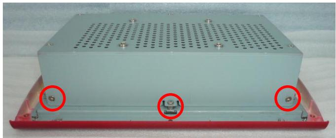
8. Lift off the metal bottom cover in the direction of the arrow.
