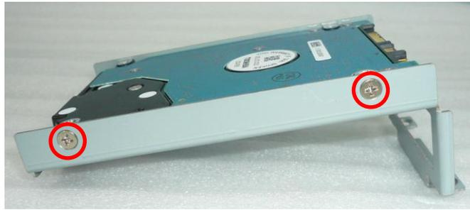
7. Insert the replacement hard disk into the HDD holder, and reattach the screws.
