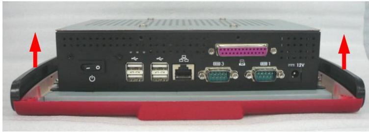
7. Remove the eight screws that secure the metal bottom cover to the main unit.
