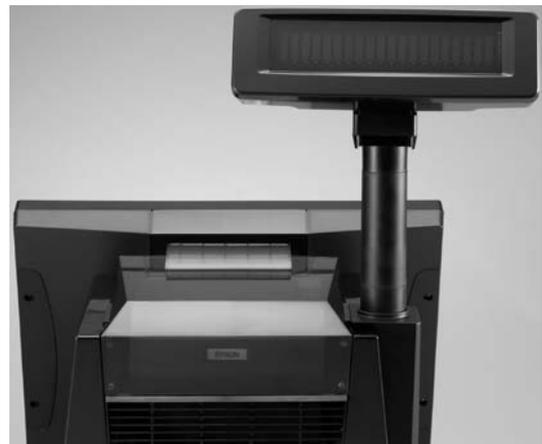
6. Only plug the cable into COM6 port when you install VFD module. Plug the cable into COM6 port and VGA port if you would like to install 8.9" LCD module.
