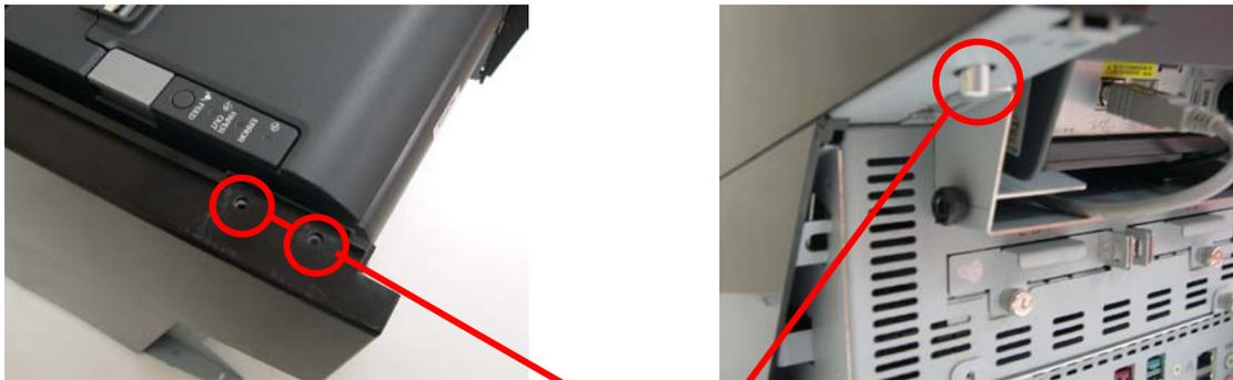
Position to screw the 2<sup>nd</sup> display module
